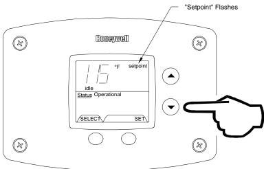
Step 5: When the desired setpoint is reached on the water heater display, press the "Set" button to confirm the new setpoint. "Setpoint" stops flashing in the water heater display.
